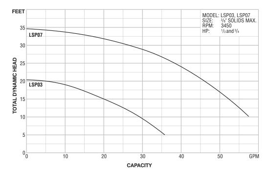
\*Vertical distance from water level to highest point in discharge – plus pipe friction.
